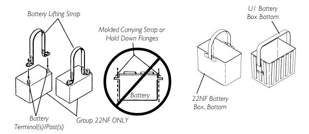
FIGURE 11.5 Installing/Removing Batteries Into/From Battery Boxes
